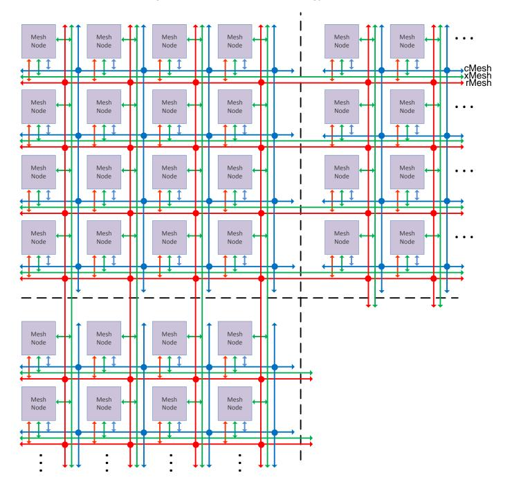
The cMesh on-chip network has significantly lower latency and higher bandwidth than the xMesh network, so tasks with significant inter-task communication should be placed together on the same chip for optimal performance.
