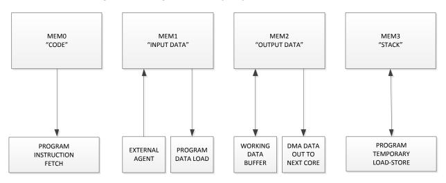
Figure 11: Program Memory Layout Optimized for Size
