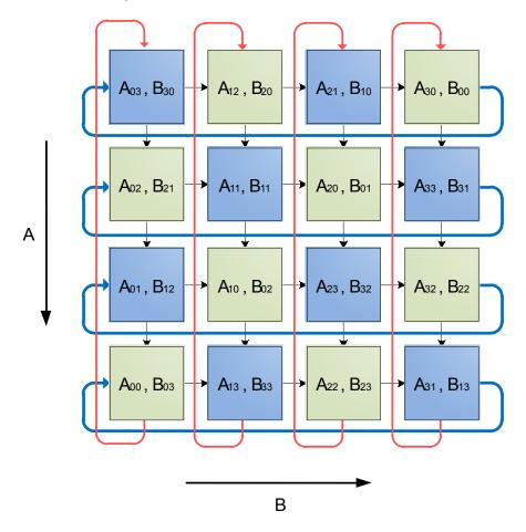
Figure 3: Matrix Multiplication Data Flow
